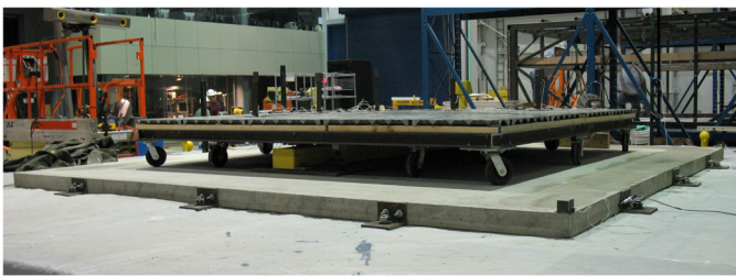
Fig. 1. Overview of isolated floor system (without wall and steel edge plates)
